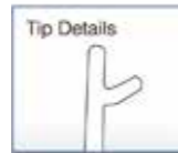
41-4007 - Haefliger Chopper Tip Angled at 45 Degrees Tip L 11mm O/L 115mm
