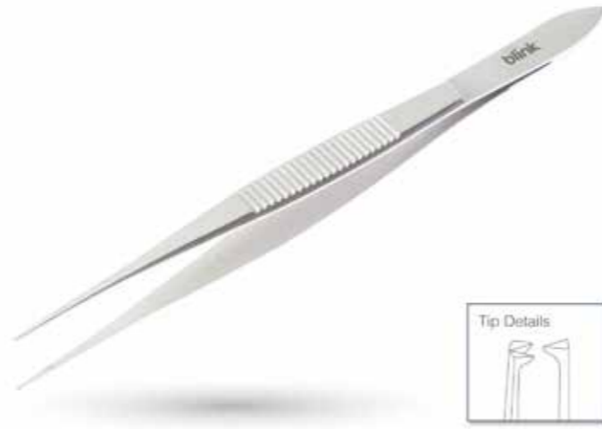
10-1302 - Forceps Utility Lister 1:2 Teeth 0.8mm with 6mm Tying Platform, O/L 114mm
