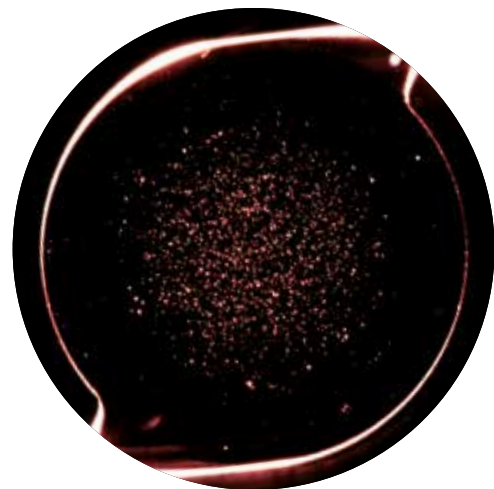
AcrySof IQ SN60WF (Alcon)* Grade 2-3, based on Miyata et al. [4] with 264.4 ± 110.3 MV/mm 2
